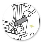
Push the check button to know the number\*\* of cartridges in the magazine.
