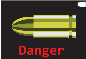
Figure 86: DCR mode screen showing there is a round detected in the chamber.
