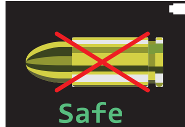
Figure 87: DCR mode screen showing there is no round detected in the chamber.
